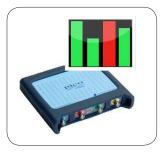
The NVH test is built into our PicoDiagnostics software. Click the icon on your Desktop and select NVH from the selection of test buttons (you have to have a PicoScope connected and an NVH license to run this test). The software will run you through a setup wizard to prepare the vehicle for a live test.
