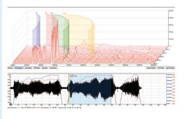
Our NVH kits use a combination of accelerometers, microphones and technical data to measure, calculate and analyze the rotating and vibrating components in a vehicle. By being able to correctly analyze the results you see on-screen, you can identify the root cause of your NVH issue.
