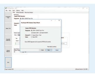
2. Input vehicle data, engine configuration, drivetrain arrangement, differential ratio, and tire size information.
